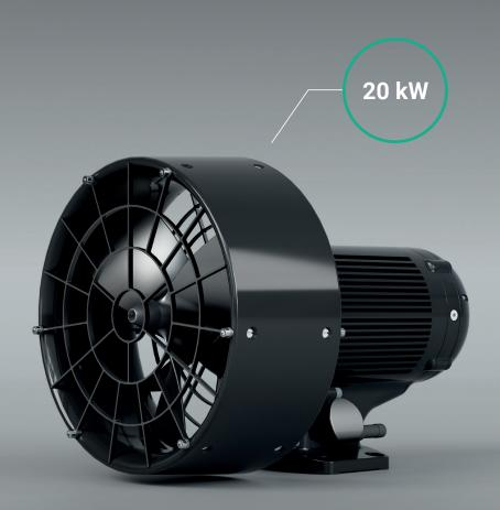
Engineered for 24/7 operation for up to 30 days without intervention. Our electric thruster delivers relentless power and durability and sets a new standard for efficiency and environmental consciousness. Featuring an integrated pressure-tolerant power inverter, fully isolated design, and dual rotary shaft seals, it exemplifies our dedication to cutting-edge engineering.
