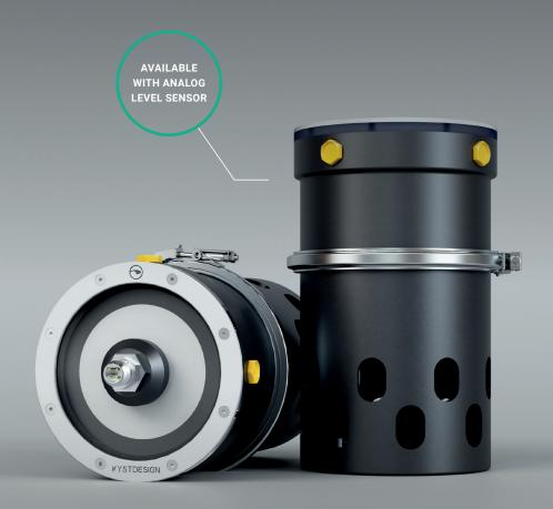
The function of the compensator is to maintain a raised pressure in a fluid circuit related to ambient at all water depths. This is achieved by a spring acting on a rolling diaphragm, i.e. the connected fluid circuit will always see a pressure equal to ambient sea water pressure plus the pressure generated by the spring.
