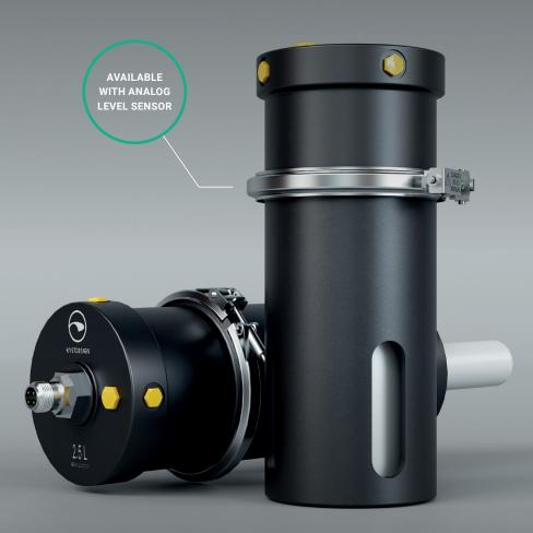
The function of the compensator is to maintain a raised pressure in a fluid circuit related to ambient at all water depths. This is achieved by a spring acting on a rolling diaphragm, i.e. the connected fluid circuit will always see a pressure equal to ambient sea water pressure plus the pressure generated by the spring.
