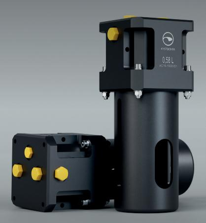
The function of the compensator is to maintain a raised pressure in a fluid circuit related to ambient at all water depths. This is achieved by a spring acting on a rolling diaphragm, i.e. the connected fluid circuit will always see a pressure equal to ambient sea water pressure plus the pressure generated by the spring.
