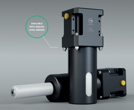
The function of the compensator is to maintain a raised pressure in a fluid circuit related to ambient at all water depths. This is achieved by a spring acting on a rolling diaphragm, i.e. the connected fluid circuit will always see a pressure equal to ambient sea water pressure plus the pressure generated by the spring.
