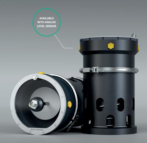
The function of the compensator is to maintain a raised pressure in a fluid circuit related to ambient at all water depths. This is achieved by a spring acting on a rolling diaphragm, i.e. the connected fluid circuit will always see a pressure equal to ambient sea water pressure plus the pressure generated by the spring.
