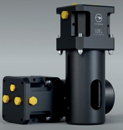
The function of the compensator is to maintain a raised pressure in a fluid circuit related to ambient at all water depths. This is achieved by a spring acting on a rolling diaphragm, i.e. the connected fluid circuit will always see a pressure equal to ambient sea water pressure plus the pressure generated by the spring.
