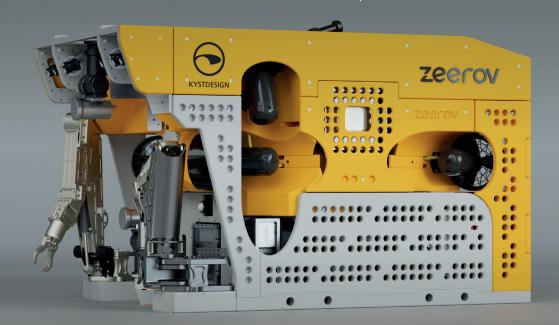
The new generation ROV, ZEEROV, is a full electric work-class ROV with an impressive power management system that gives the ROV increased power and better maneuverability within the same size as the successful Supporter ROV. The ZEEROV is designed with a high focus on reliability and flexibility which is the key success factor for achieving long term submersion and effective remote control from shore.
